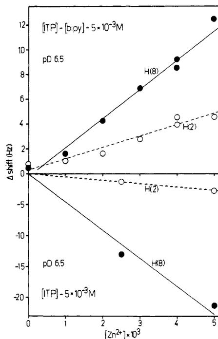
**Figure 3.** Change in chemical shift,  $\Delta$  shift, of the  $^1\text{H}$  NMR resonances for H(2) and H(8) of ITP in the presence (upper part) and absence (lower part) of 2,2'-bipyridyl in  $\text{D}_2\text{O}$  at pD 6.5 in dependence on  $[\text{Zn}(\text{ClO}_4)_2]$ ;  $[\text{ITP}] = 5 \times 10^{-3} \text{ M}$  ( $= [\text{bpy}]$ , if present); 25 °C. The chemical shifts of free ITP at pD 6.5 are 762 Hz for H(8) and 739 Hz for H(2).
